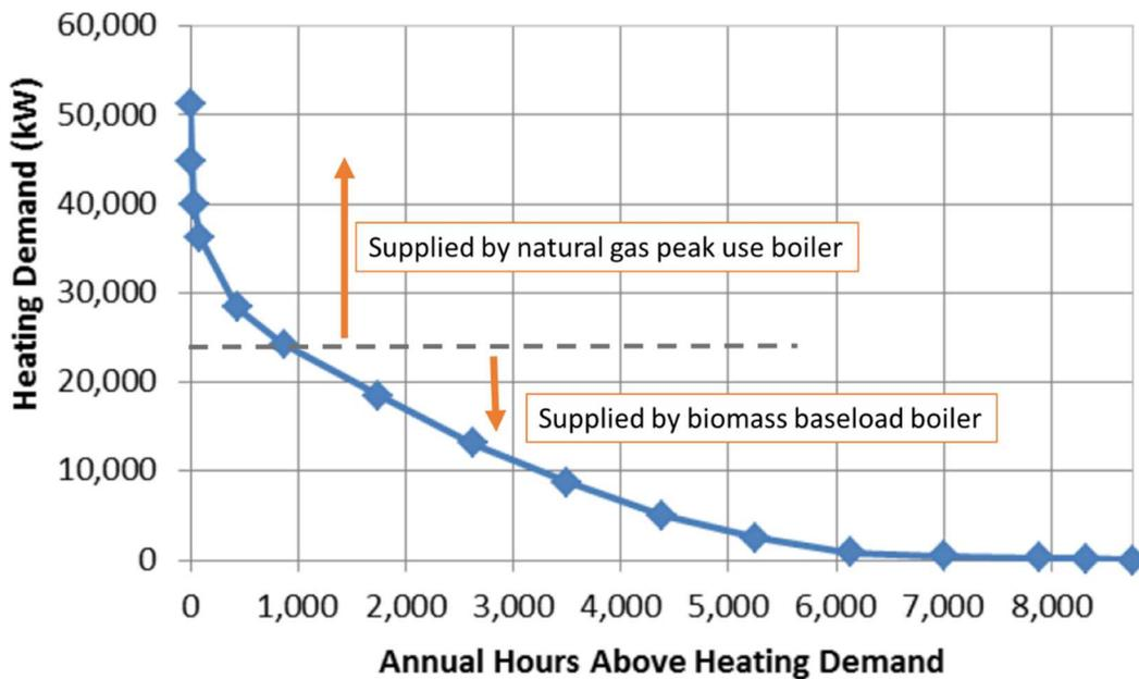
A CHP supply may be an attractive option for a baseload supply, based on the combustion of NG, biomass or other fuel. The combustible fuel is used to drive a generator and produce electricity, which may be used onsite to offset the amount of electricity purchased. The waste
