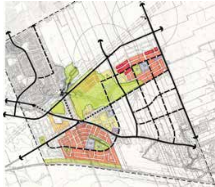
Figure 17: This figure illustrates the interim and ultimate collector and arterial road network. Short dotted lines show connections, from Renaud and Pagé Roads, to Navan Road that will remain open until such time as alternative connections exist. Dashed lines represent the future local collector network. Solid lines show the major north-south and east-west routes (such as Mer Bleue Road, Navan Road, the future Belcourt Extension, the future Blackburn Hamlet By-pass and Orléans Blvd.)
