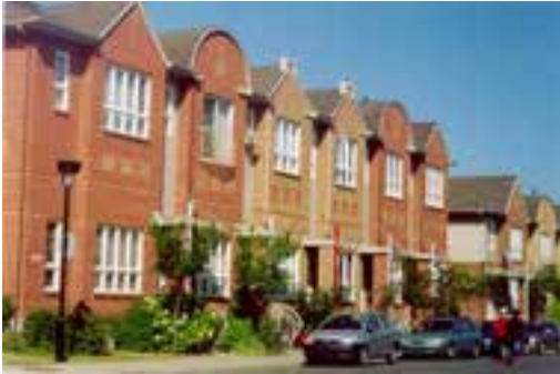
Figure 41: Varied brick colours and small setbacks help to reduce the impression of one long continuous wall.
