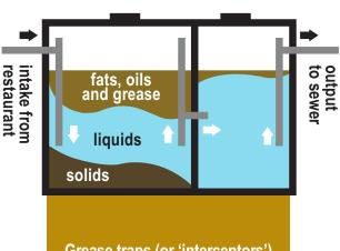
Grease traps (or 'interceptors') are designed to trap fats, oils and grease and can help extend the life of your septic system if properly sized, installed and maintained.
