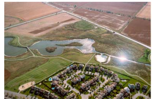
A constructed wetland in Kanata provides stormwater management and community pathways.
