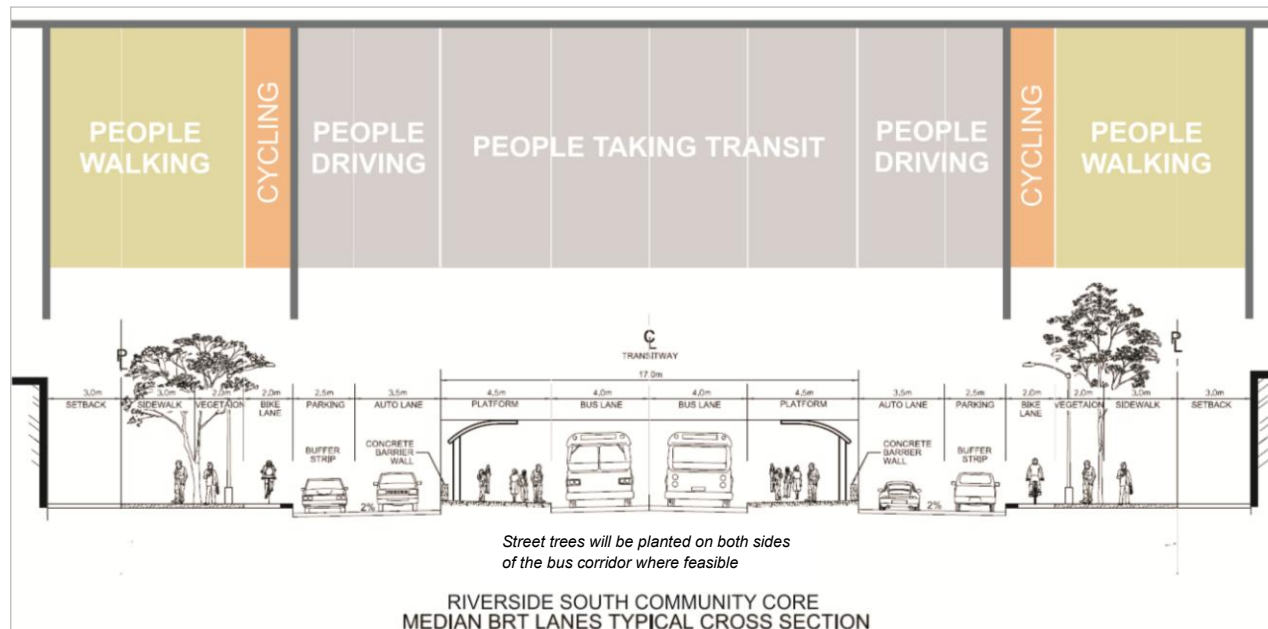
Figure 20: Transit Street Cross-Section with Median BRT Lanes in Riverside South Community Core
