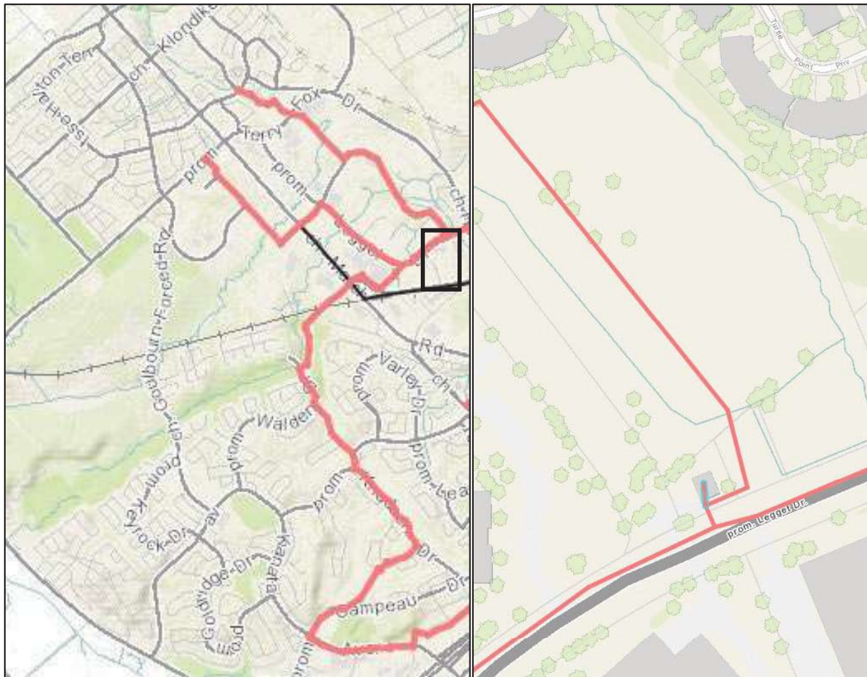
Figure 1 - Map of the March Road pumping station and its two incoming wastewater lines from the North and West and outgoing to the East. Right image is a zoom in of the area marked by the box on the left image. Cyan blue highlights the exact location measured by the flow probe.
