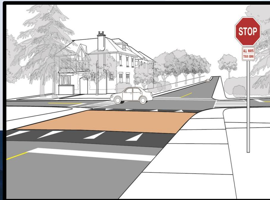
**Cycle-friendly bulb-outs** are horizontal projections of curbs into roadways that includes spaces for cyclists to ride over or through it
